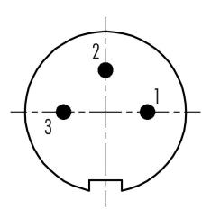
Contact arrangement (Plug-in side)
