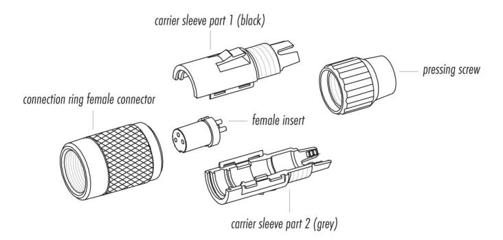
Attention: max. torque of ring nut in socket connector: 50cNm (manual adjustment)
