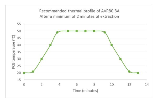
This thermal profile can be adapted:  $\pm 10^{\circ}$ C, depending some more parameters, such as: thickness deposit, design of the PCB...
