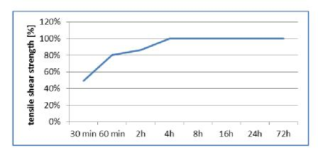
compression shear strength shaft-hub joint with activator DELO-QUICK 5006 based on initial value at room temperature measured at room temperature (approx. 23 ℃) according to ISO 10123
