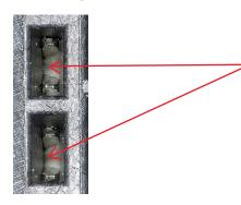
The tips of the insulation displacement contacts that were pushed into the cable need to be visible through the inspection window on the underside of the IDC connector.
