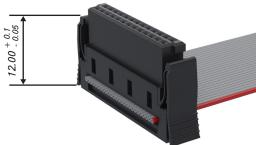
Inspecting this dimension is important because it allows employees to determine whether the connector is compressed enough to be securely locked in this position.
