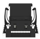
The cable duct on the IDC bridge needs to be free – in other words, the insulation displacement contacts cannot be inside the cable duct. This ensures that the cable can be securely routed through the duct.
