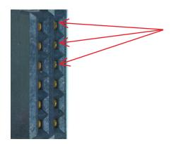
When the connected depth is correct, a small air gap (specification: min. 0.1 mm) is visible between the top of the contact tongue and the insulator material.
