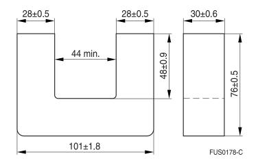
The A<sub>I</sub> value in the table applies to a core set comprising two ungapped cores.
